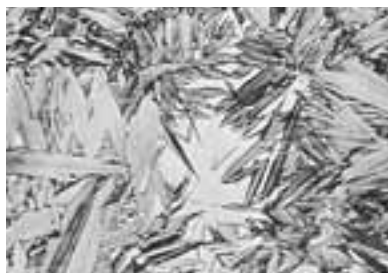
Photomicrograph of martensite.
