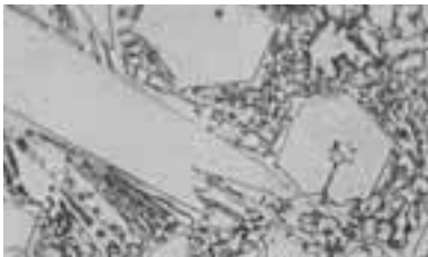
Photomicrograph of large carbides in a carbide eutectic matrix.
