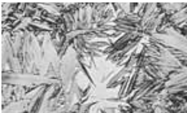
Photomicrograph of martensite.
